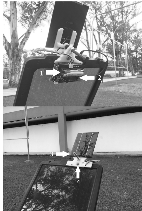
Fig. 5. Physical setup: (1) Battery, (2) electrical parameters sensor, (3) auxiliary PV panel, (4) luxometer on top and temperature/humidity sensor on bottom.
